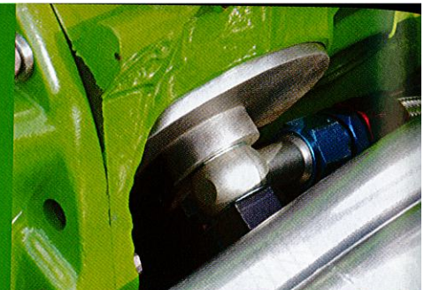
Richard fabricated a remote oil filter and cooler system to solve clearance issues.
