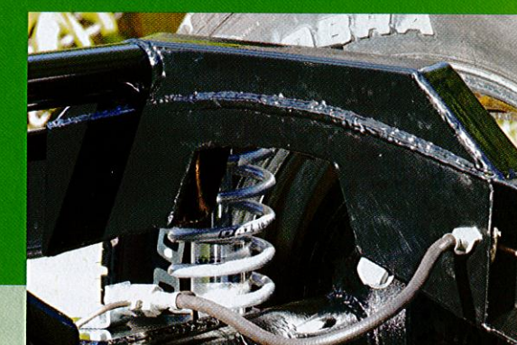
Above and above right > Richard fabricated the four-link rear. Lee had already c-notched the chassis.
